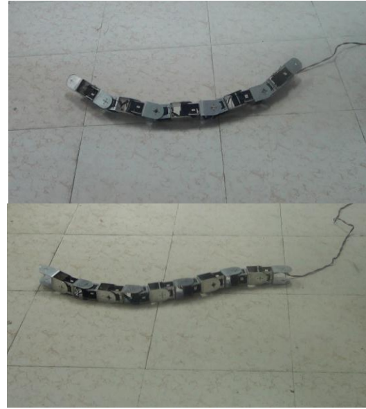
Fig.4. shows rolling motion on a flat surface (top); sidewinding motion on a flat surface (bottom).
